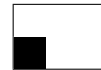
Figure 9: A room of 3 by 2 where the left lower cell can be used by another room. White is closed and black is open.
